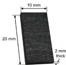
Fig. 1. Shape and dimensions of the magnetite specimen.
