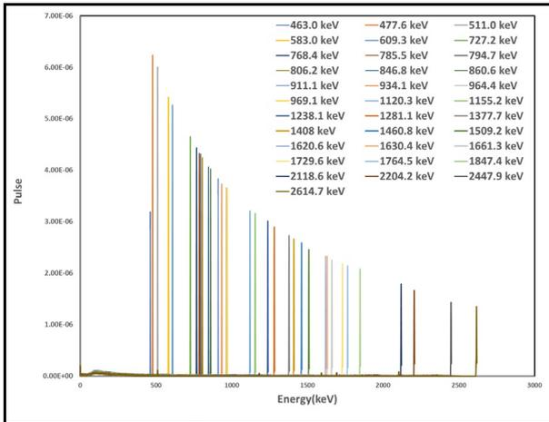
Fig. 2. Gamma spectra of natural nuclides calculated by MCNP simulation
