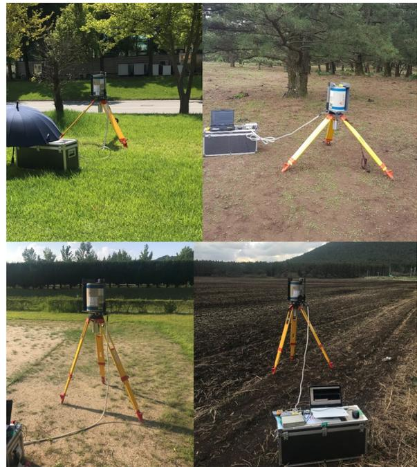
Fig. 1. In-situ gamma-ray spectroscopy for measurement of natural nuclides at sites.
