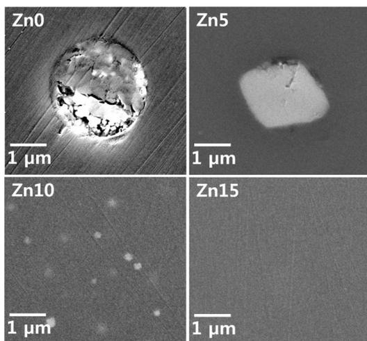
Fig. 2. SEM images of the cross-section of  $\text{Mo}_2\text{Zn}_X$  series glasses slowly cooled at  $1^\circ\text{C}/\text{min}$ .
