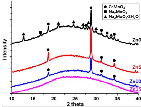
Fig. 1. XRD patterns of  $\text{Mo}_2\text{Zn}_X$  series glasses slowly cooled at  $1^\circ\text{C}/\text{min}$ .
