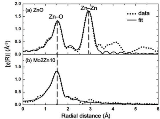
Fig. 3. The Fourier-transformed EXAFS from (a) ZnO and (b)  $\text{Mo}_2\text{Zn}_{10}$  as a function of the distance from a Zn atom. The dotted lines show the experimental data and the solid lines are the fits.
