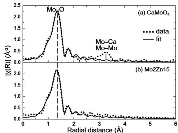
Fig. 4. The Fourier-transformed EXAFS from (a)  $\text{CaMoO}_4$  and (b)  $\text{Mo}_2\text{Zn}_{15}$  as a function of the distance from a Mo atom. The dotted lines show the experimental data and the solid lines are the fits.
