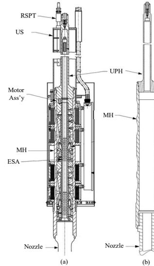
Fig. 1. Control element drive mechanism (CEDM): (a) all components, (b) pressure boundary components.
