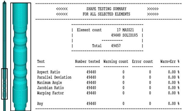
Fig. 2. Full FE model of the CEDM and mesh check result.
