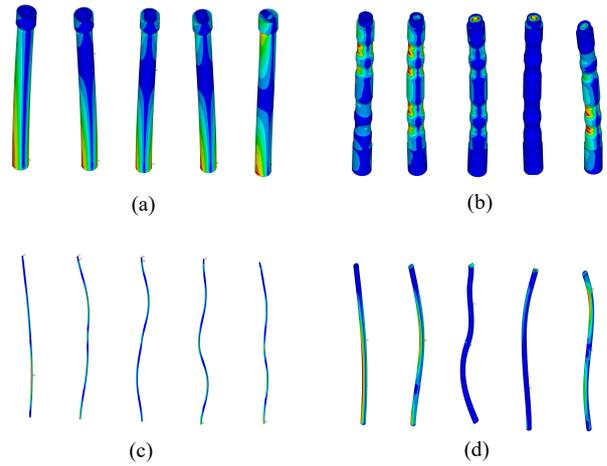
Fig. 3. Von-Mises stress results from first five modes of modal analysis results: (a) nozzle, (b) motor housing, (c) upper pressure housing, (d) upper shroud.
