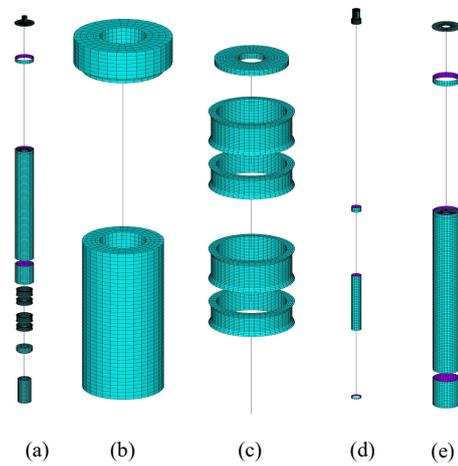
Fig. 4. Hybrid FE model of the CEDM: (a) CEDM, (b) nozzle, (c) motor housing, (d) upper pressure housing, (e) upper shroud.
