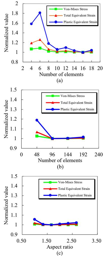
Fig. 6. Mesh sensitivity results with varying number of elements in (a) the thickness (radial) direction and (b) the rotational (circumferential) direction and (c) the aspect ratio.
