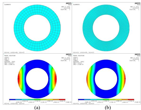
Fig. 7. Equivalent plastic strain results: number of elements in the thickness, the circumferential direction, aspect ratio; (a) (4, 16, 1.3), (b) (16, 96, 1.6)
