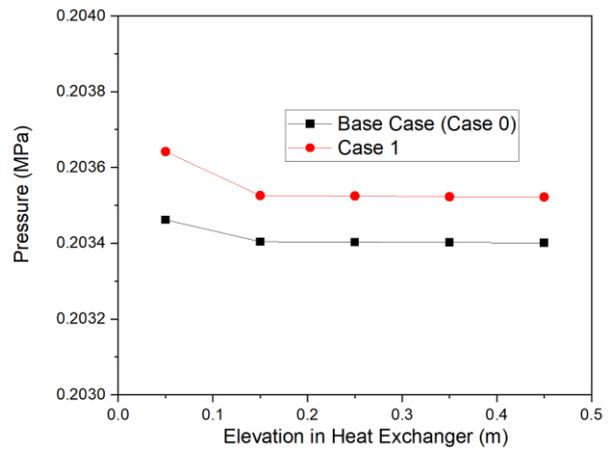
Fig. 2. Pressure distribution in the heat exchanger
