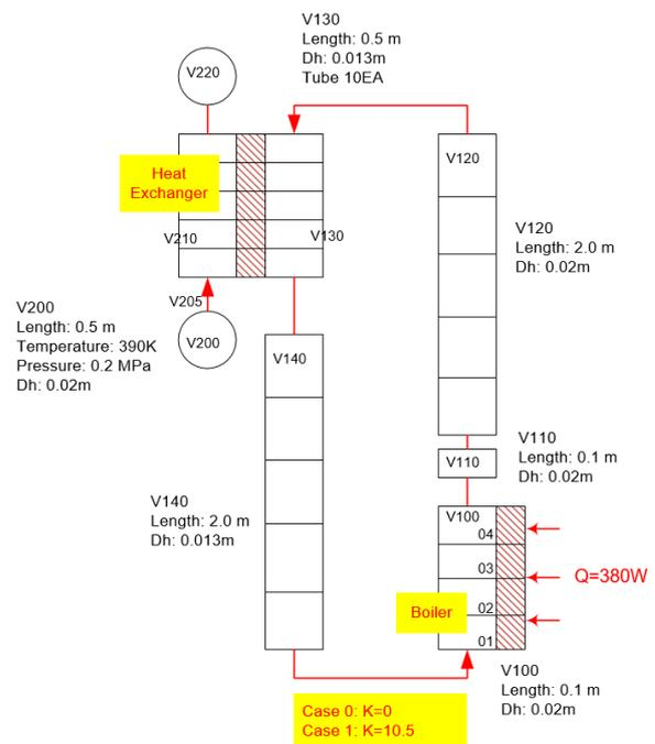
Fig. 1. MARS model for conceptual heat exchanging system
