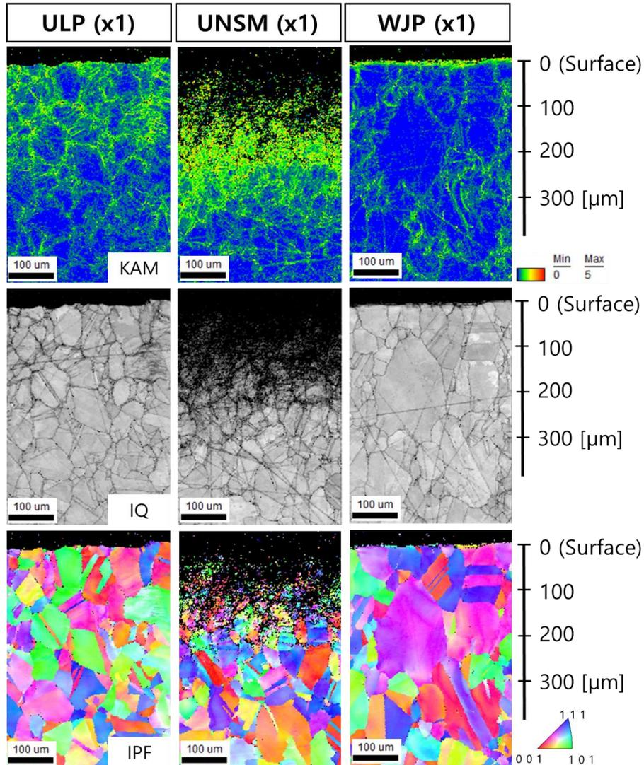
Fig.5. EBSD microstructure analysis result of one-time peened specimen.
