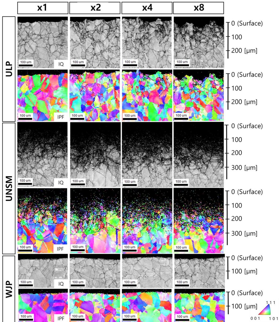
Fig.6. EBSD microstructure analysis result of the over peened specimen.
