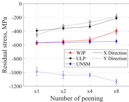
Fig. 3. XRD surface residual stresses of over-peened specimens depending on peening methods.
