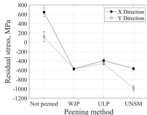
Fig. 2. XRD surface residual stresses of specimens depending on peening methods.
