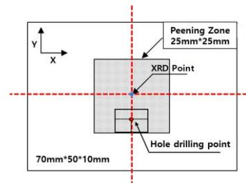
Fig. 1. Schematic of alloy 600 peening specimen surface; x-direction: grinding and peening process direction, y-direction: peening step direction.
