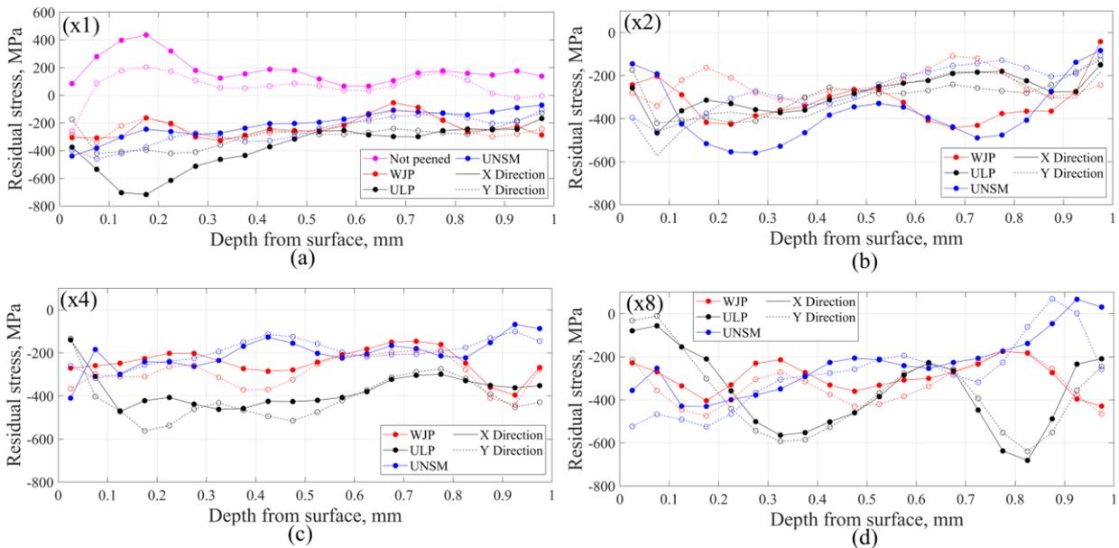
Fig. 4. The hole drilling depth-profiling residual stress results. (a) single peening results, (b) 2-times peening results, (c) 4-times peening results, (d) 8-times peening results.
