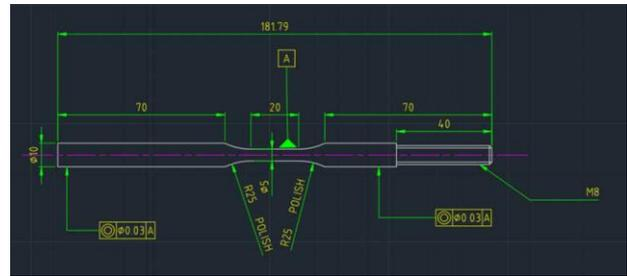
Fig. 1. High-speed tensile test specimen (mm)
