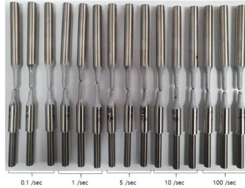
Fig. 3. Specimens after high-speed tensile tests
