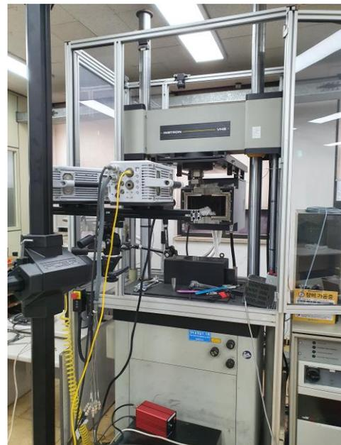
Fig. 2. High-speed tensile test facility
