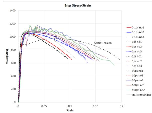
Fig. 4. Stress-strain curves of SNB7 for various strain rates
