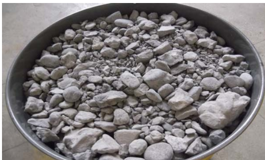
Figure 1. Decommissioning Concrete Waste Drum
