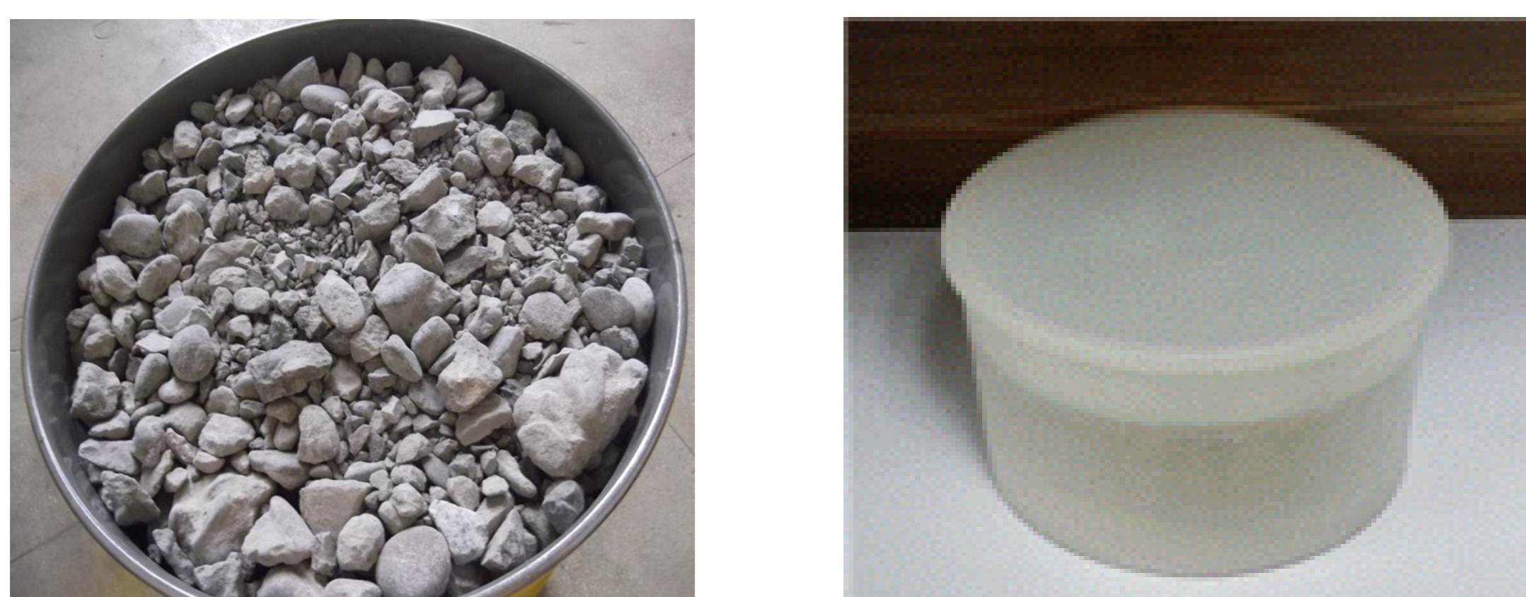
Figure 1. Decommissioning Concrete Waste Drum & Sampling material
