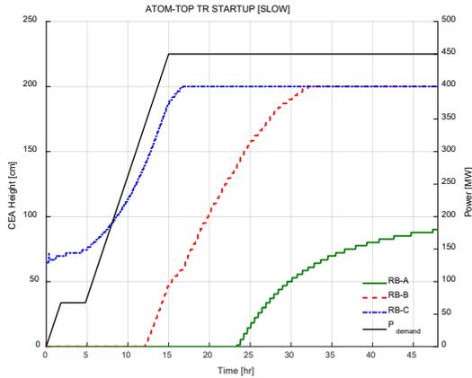
Figure 7. CEA position during startup
