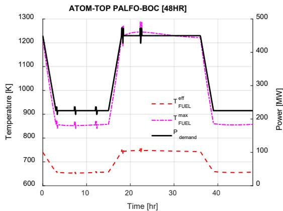
Figure 13. Doppler fuel temperature profile during PALFO
