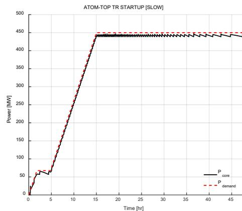
Figure 6. Core power vs. Demand power during startup
