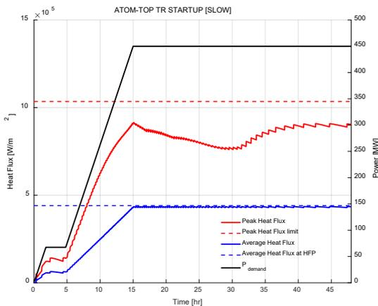
Figure 9. Heat flux profile during startup
