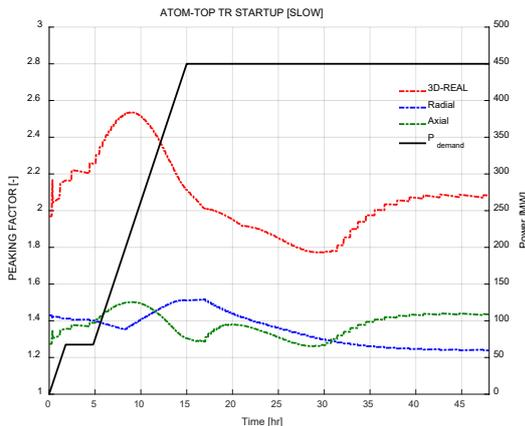
Figure 8. Power peaking profile during startup
