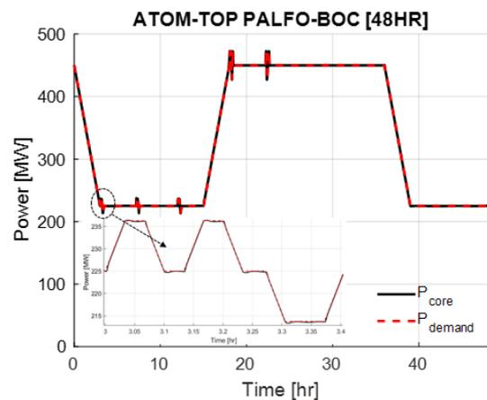
Figure 10. Core power vs. Demand power during PALFO
