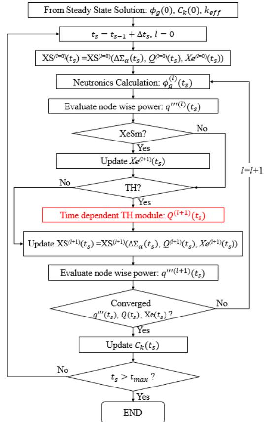
Figure 1. Calculation flowchart of KNS3D
