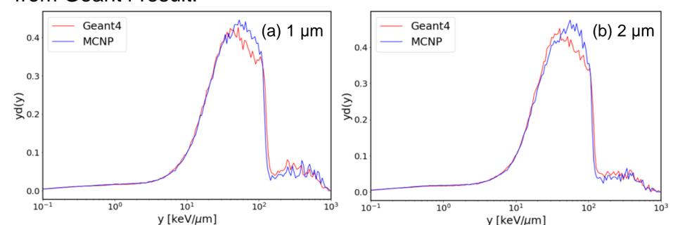
**Fig. 4.** Dose distribution spectrum of <sup>252</sup>Cf simulation for the simulated tissue sizes 1 and 2 μm.
