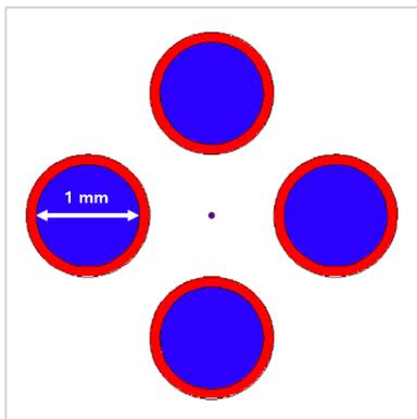
**Fig. 1.** Four identical detectors surrounding the point source in the middle point. The blue circle is the propane-based TE gas and the red ring is the A-150 TE plastic.
