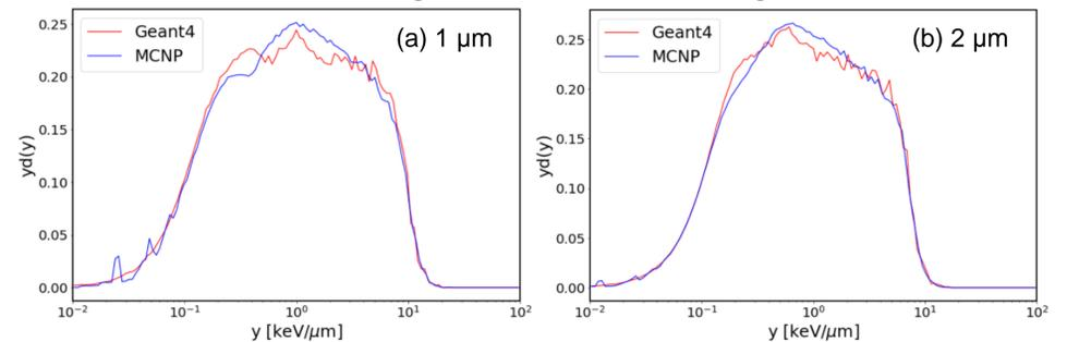
**Fig. 3.** Dose distribution spectrum of <sup>137</sup>Cs simulation for the simulated tissue sizes 1 and 2 μm.
