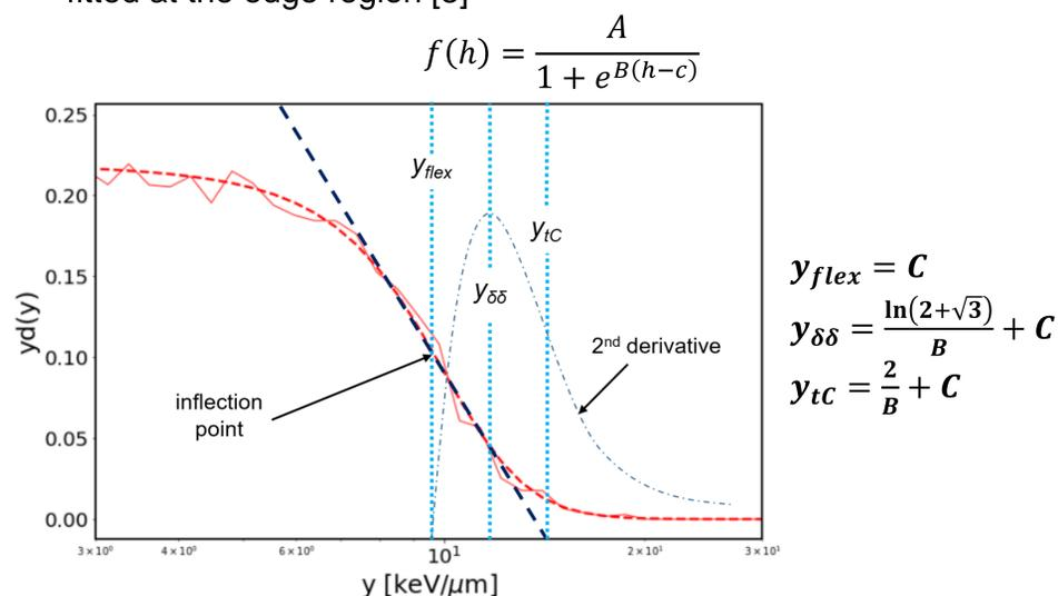
**Fig. 2.** Three possible calibration points in  $yd(y)$  spectrum
