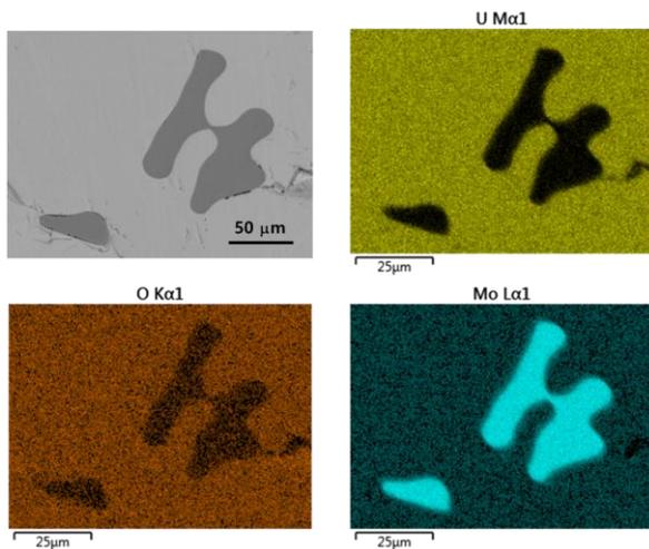
Fig. 3. SEM and EDS elemental mapping images at the selected area of sample annealed at 2730°C
