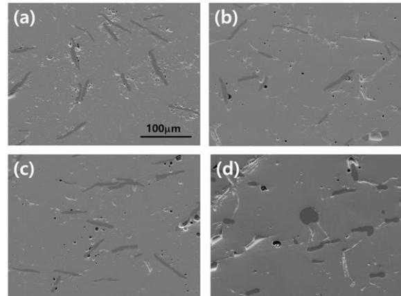
Fig. 1. SEM microstructures of UO<sub>2</sub>-Mo pellets; (a) as-fabricate, and annealed at (b) 2530°C, (c) 2670°C, and (d) 2730°C
