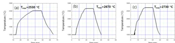
Fig. 2. Annealing temperature profiles. (a) T<sub>max</sub>=2530°C, (b) T<sub>max</sub>=2670°C, (c) T<sub>max</sub>=2730°C
