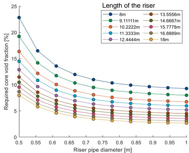
**Figure 5.** Required core void fraction to achieve the reactor power of 200MW<sub>t</sub> (two-phase).
