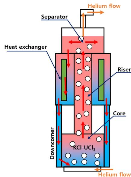
Figure 1. A schematic of the natural circulating PMFR
