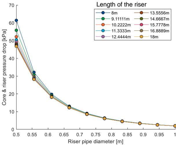
**Figure 3.** Frictional pressure loss of the core and riser with helium injection (two-phase).
