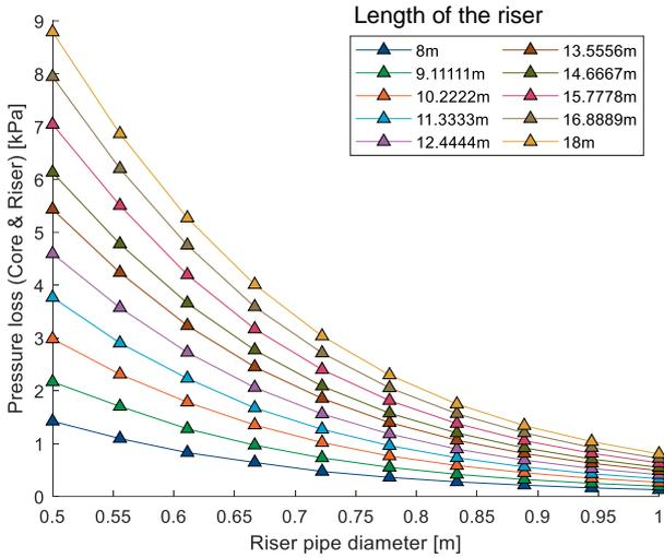
**Figure 2.** Frictional pressure loss of the core and riser without helium injection (single phase).
