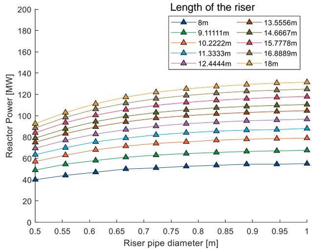
**Figure 4.** Achievable powers without helium bubbling (single phase).
