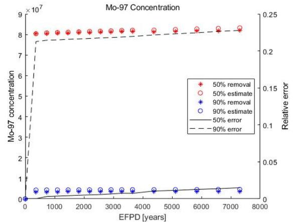
Figure 4. Molybdenum-97 concentration as a representative of removed noble metal
