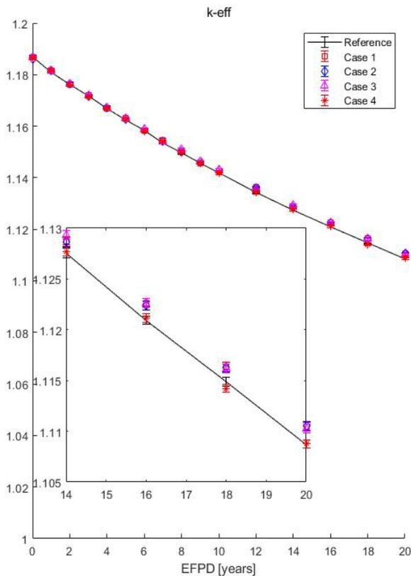
Figure 2.  $k_{\text{eff}}$  comparison between reference and removal test cases with different removal efficiencies. Error plotted with  $2\sigma$
