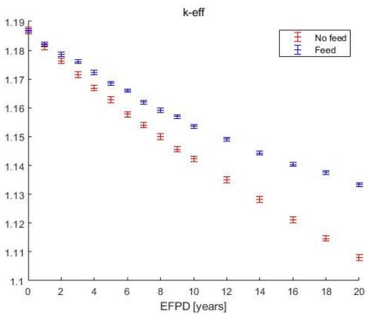
Figure 5. k-eff comparison between reference and continuous refueling. Error plotted with  $2\sigma$
