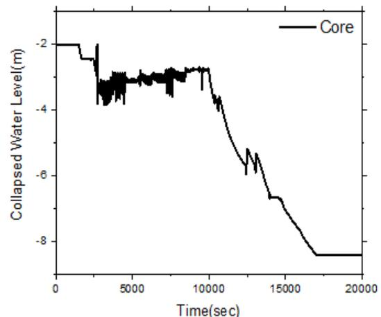
Fig. 3. Collapsed Water level of the core.
