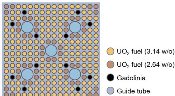
Figure 3. B1 type fuel assembly of APR1400 problem
