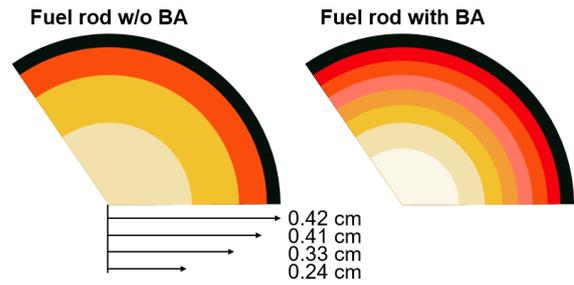
Figure 4. Geometry of fuel rods for fuel depletion
