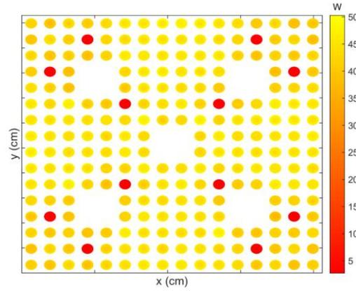
Figure 7. Intra pin power distribution at 0 EFPD (iDTMC)
