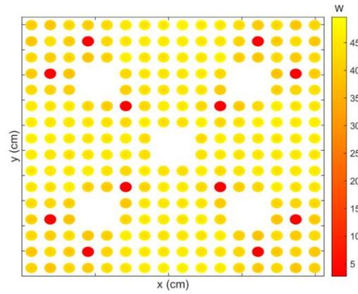
Figure 6. Intra pin power distribution at 0 EFPD (MC)
