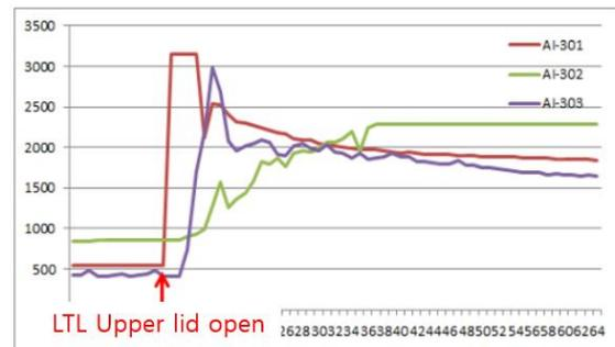
Fig. 1. The oxygen concentration changes without purging.
