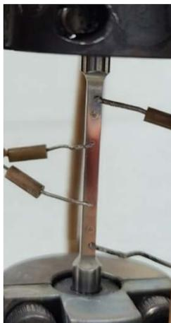
Fig. 2. Platinum probe which supplies direct current and measures potential drop
