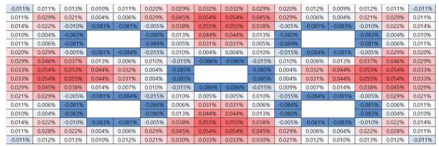
Fig. 6. Power Distribution Error between 20  $\mu\text{m}$  coated and base Assembly [A0 Assembly]
