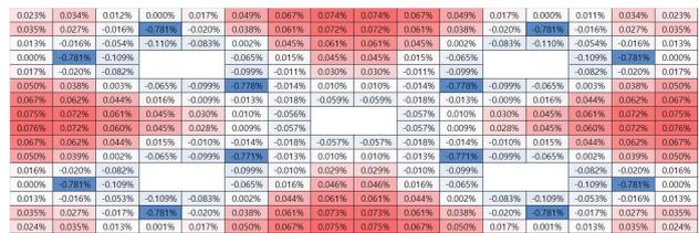
Fig. 8. Power Distribution Error between 20  $\mu\text{m}$  coated and base Assembly [B2 Assembly]
