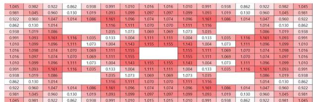
Fig. 7. Power Distribution with 20  $\mu\text{m}$  coated B2 Assembly
