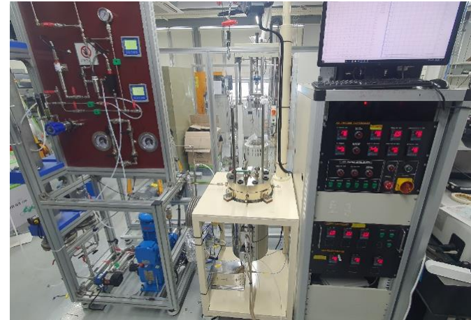
Fig. Accelerated corrosion loop system
