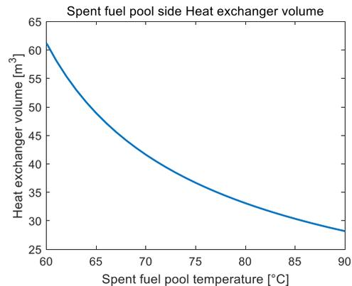
Fig. 4. Spent nuclear fuel pool side Heat exchanger volume according to the target pool temperature
