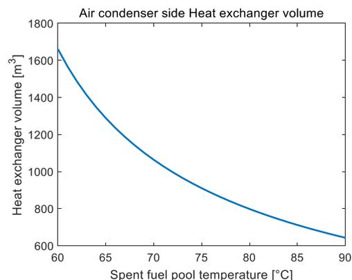
Fig. 5. Air condenser side Heat exchanger volume according to the target pool temperature
