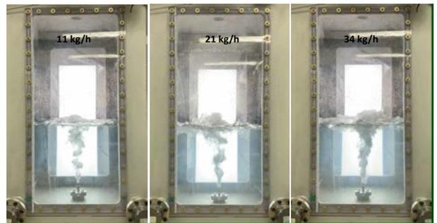
Fig. 4. Pool scrubbing experiments with injection gas flow rate.
