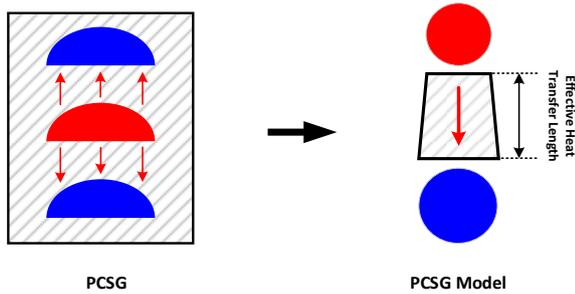
Fig 3. Schematic drawing of the effective heat transfer length for the PCSG model
