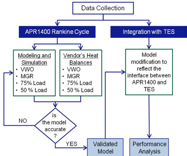
Fig.2. Model development methodology flow diagram
