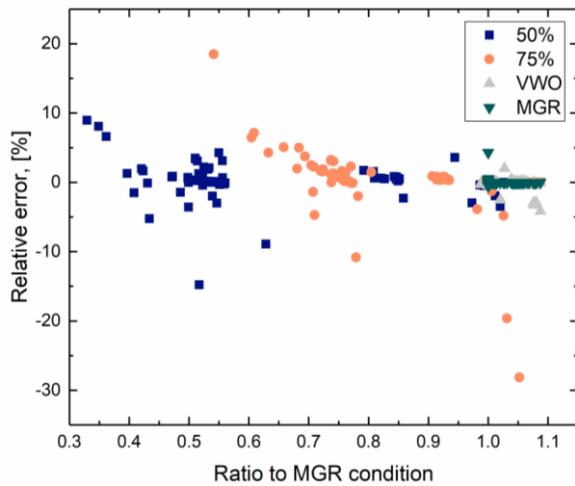
Fig.4. Relative error plotted against a ratio of flow parameters (mass flow rates, pressures and enthalpies) at given condition to their values at nominal condition.
