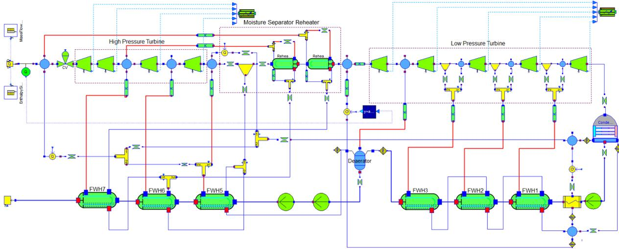
Fig.3. APR1400 secondary system model developed in OMEdit
