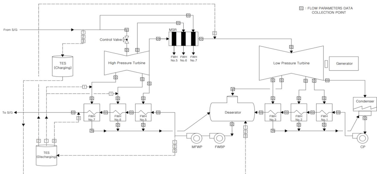
Fig.1. Simplified diagram of the APR1400 secondary cycle integrated with three different configurations of TES interface (numbered 1, 2, and 3) for storage charging and discharge operation (dashed lines indicate the TES interface pipelines).
