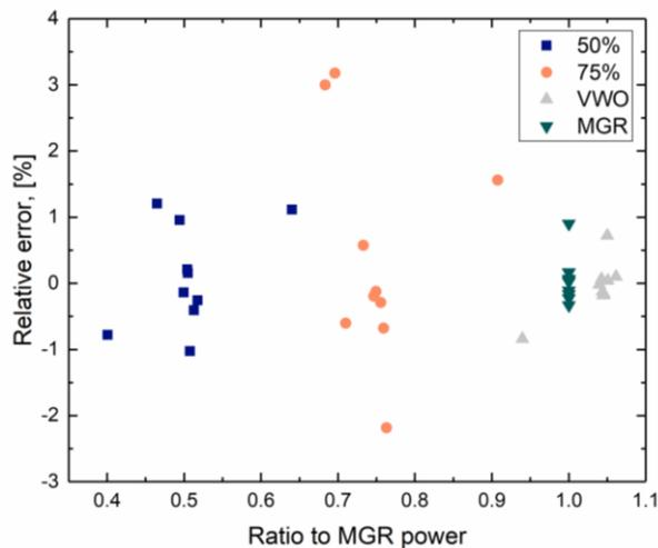
Fig.5. Relative error plotted against a ratio of turbine-generator power values (stage groups shaft power and generator power output) at given condition to their values at nominal condition.
