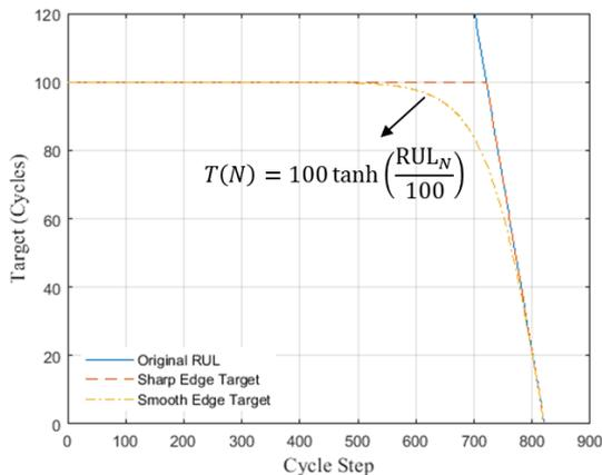
Fig. 3. Example of cycle-series target (specimen: MAH651-2).
