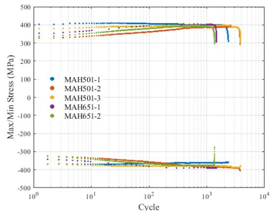
Fig. 2. Cyclic-series maximum/minimum stresses.
