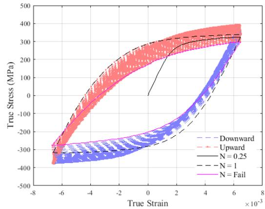
Fig. 1. Example of time-series fatigue data as represented in hysteresis loop form (specimen: MAH651-2).
