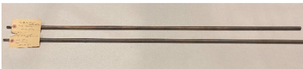
Fig. 1 Manufactured sodium heat pipes with hybrid wick structures
