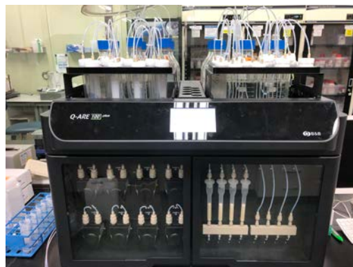
Fig. 1. Automated radionuclide extraction system (Q-ARE)
