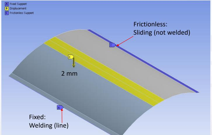
Only one edge is fixed and the other edge is slide freely along the inner cylinder surface to prevent excessive stress.
