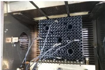
(b) Installation of specimen in the high temperature furnace
