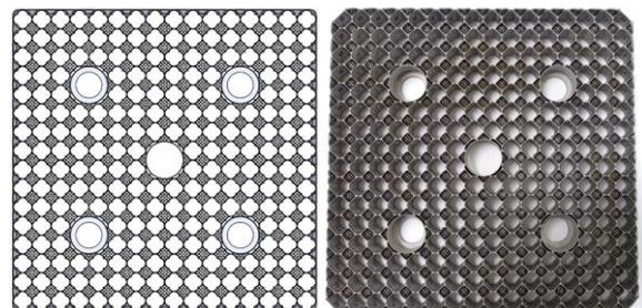
Fig. 3. 3D model (left) and actual printed (right) DFBG prototype
