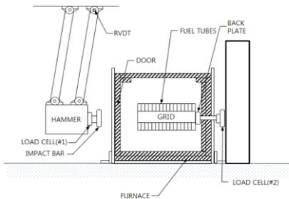
(a) Schematic of the dynamic impact test equipment
