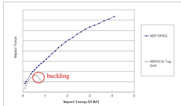
Fig. 5. Dynamic crush test result (crush strength)
