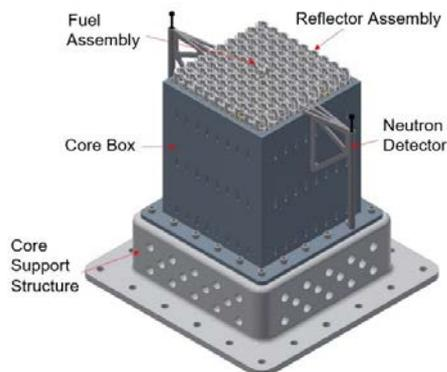
Fig. 1. Reactor Structure Assembly
