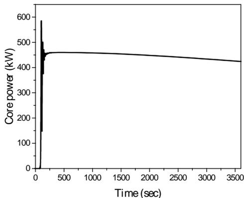
Fig. 4. Core Power in Inadvertent Withdrawal of CARs
