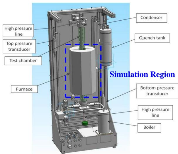
Apparatus of NRC-Studsvik test
