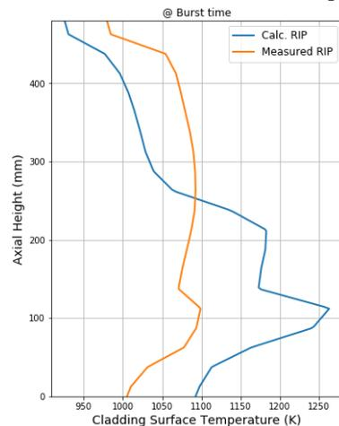
Fig. 5 Cladding surface temperature at the time of rupture
