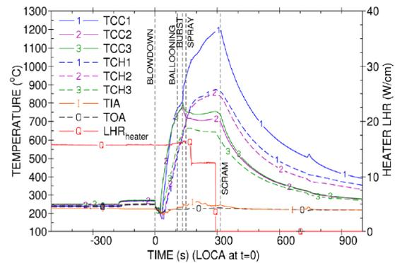
Fig. 1 Cladding and heater power in IFA-650.9 test [4]
