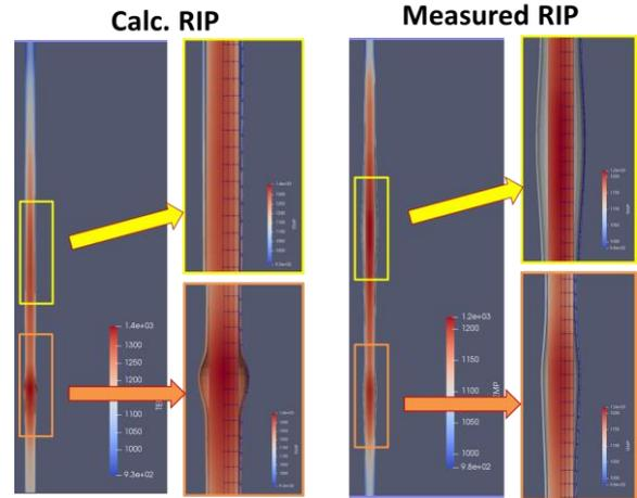
Fig. 4 Fuel temperature and deformation shape at the time of rupture.
