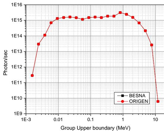
Fig. 5. Comparison of photon emission spectra obtained with BESNA and ORIGEN-S
