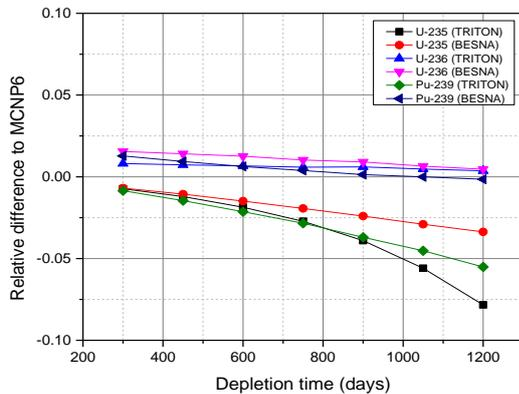
Fig. 1. Relative difference compared to MCNP6 of  $^{235}\text{U}$  and  $^{239}\text{Pu}$
