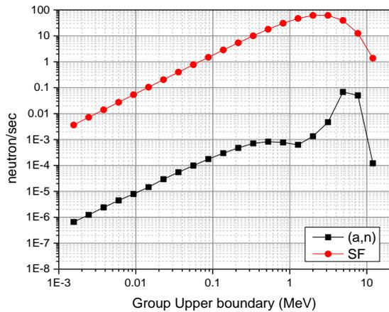
Fig. 4. Neutron spectrum from  $(\alpha, n)$  reaction and spontaneous fission for BESNA
