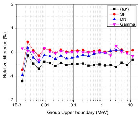
Fig. 6. Relative percent differences (%) in neutron and photon spectra between BESNA and ORIGEN-S
