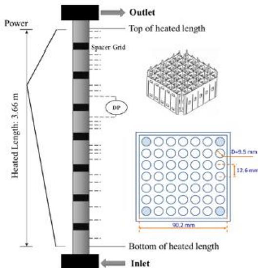
Fig. 1. Test section of RBHT facility [1].
