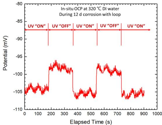
Figure 4. In-situ OCP change Zircaloy-4 with UV irradiation at 320 °C DI water
