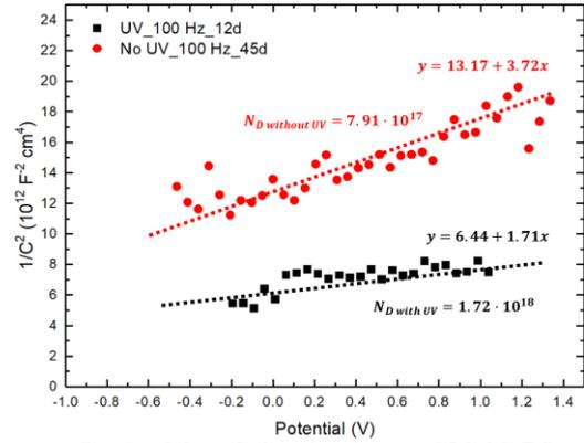
Figure 6. In-situ Mott-Schottky data at 320 °C DI water
