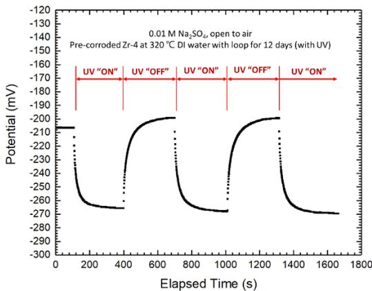
Figure 5. OCP change of 12 d UV-irradiated Zircaloy-4 at 0.01 M Na<sub>2</sub>SO<sub>4</sub> solution
