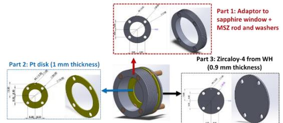
Figure 1. Advanced in-situ EIS cell design for sapphire engineered autoclave
