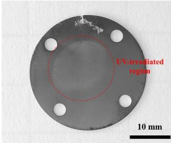
Figure 3. An optical image of UV-irradiated Zircaloy-4 for 12 d at 320 °C DI water
