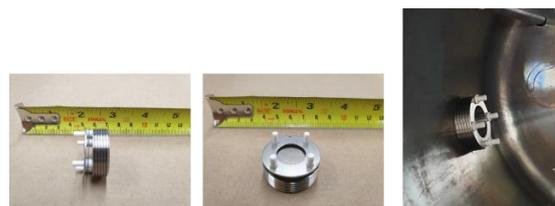
Figure 2. The compromised cell (Pt and Zircaloy-4 disk, adaptor for the autoclave)
