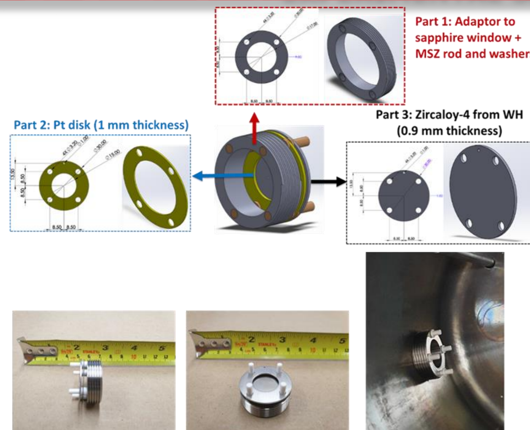
Schematic and pictures of in-situ EIS cell for sapphire window engineered autoclave
