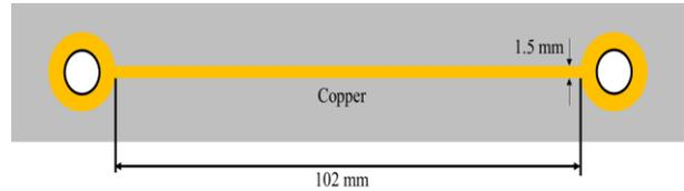
Fig 2. PCB heater
