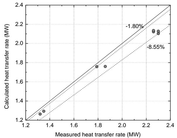
Fig. 9. Validation of heat transfer rates in PFBR FHX.
