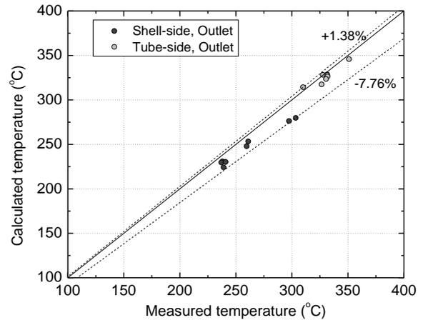
Fig. 8. Validation of outlet temperatures in PFBR FHX.
