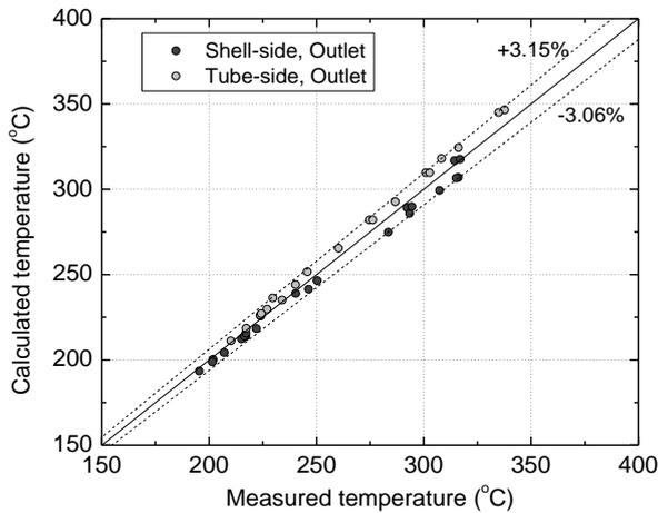
Fig. 11. Validation of outlet temperatures in SELFA FHX.
