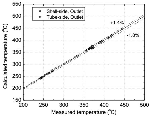
Fig. 5. Validation of outlet temperatures in JOYO IHX.
