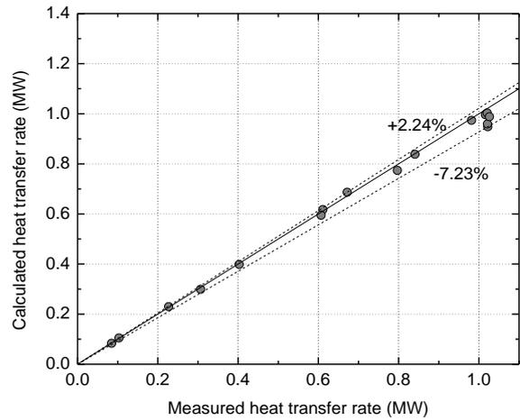
Fig. 3. Validation of heat transfer rates in STELLA-1 DHX.
