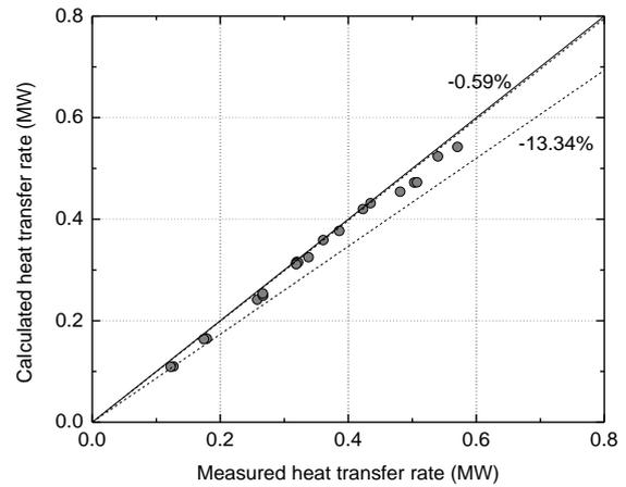
Fig. 12. Validation of heat transfer rates in SELFA FHX.
