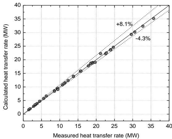
Fig. 6. Validation of heat transfer rates in JOYO IHX.
