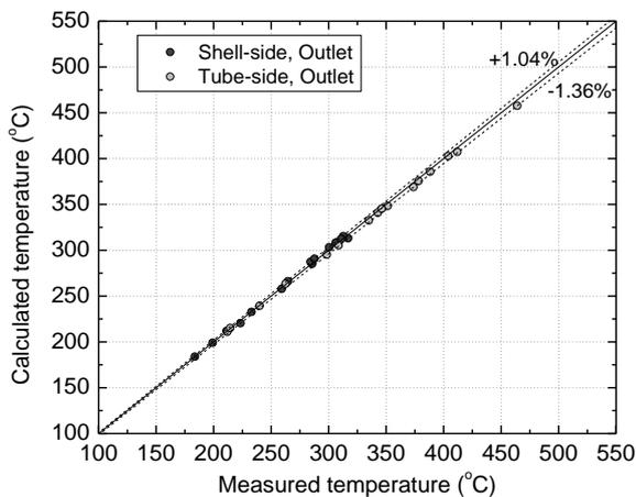
Fig. 2. Validation of outlet temperatures in STELLA-1 DHX.
