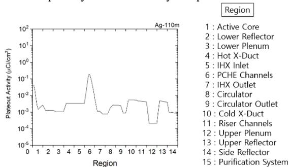
Fig. 3. Predicted plateout activity distribution of Ag-110m in the primary circuit after 40-year operation.
