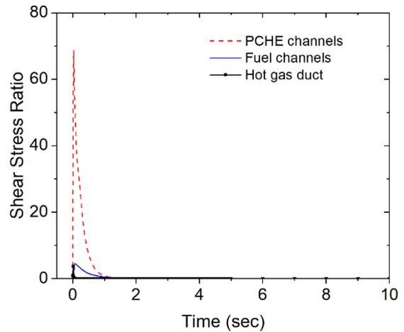
Fig. 5. Calculated shear stress ratio during depressurization accident.
