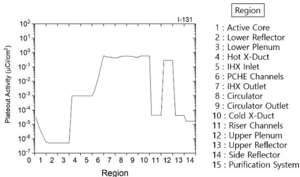
Fig. 4. Predicted plateout activity distribution of I-131 in the primary circuit after 40-year operation.
