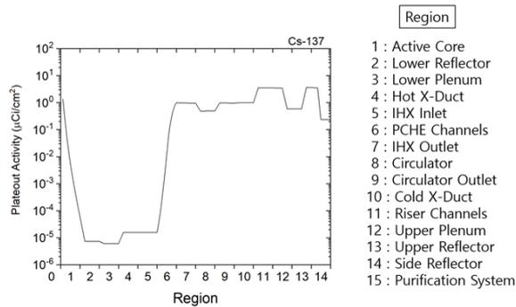
Fig. 2. Predicted plateout activity distribution of Cs-137 in the primary circuit after 40-year operation.
