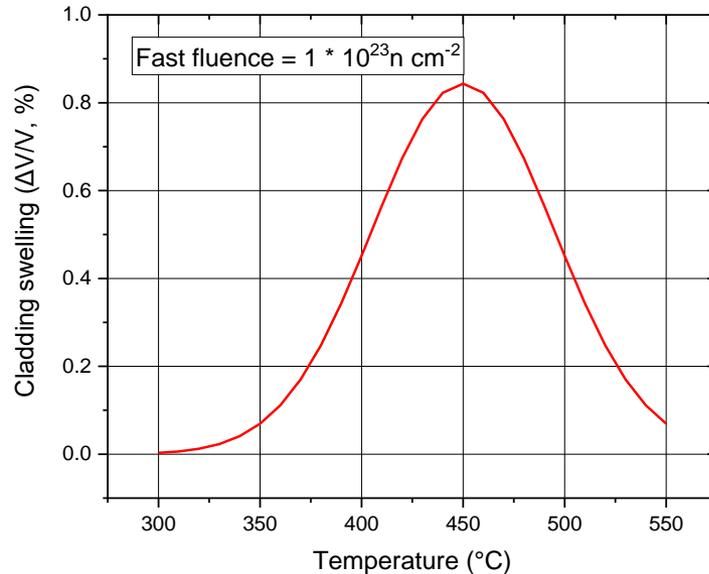
$$\frac{\Delta V}{V} [\%] = 1.5 \times 10^{-3} \exp \left[ -2.5 \left( \frac{T[^\circ\text{C}] - 450}{100} \right)^2 \right] \phi^{2.75}$$
