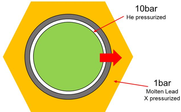
Schematic cross section image of the fuel rod
