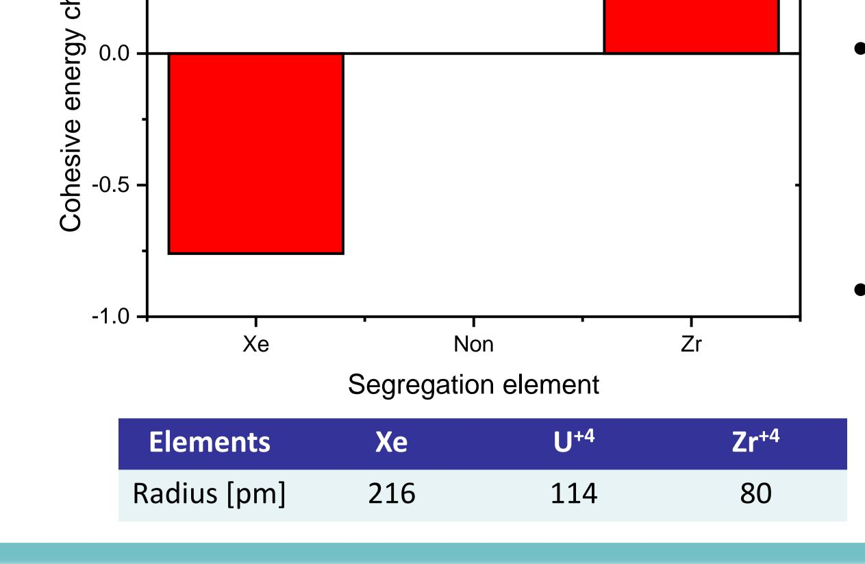
The grain boundary cohesive energy of the structure in which the zirconium was segregated was rather increased when compared to the case without segregation.
