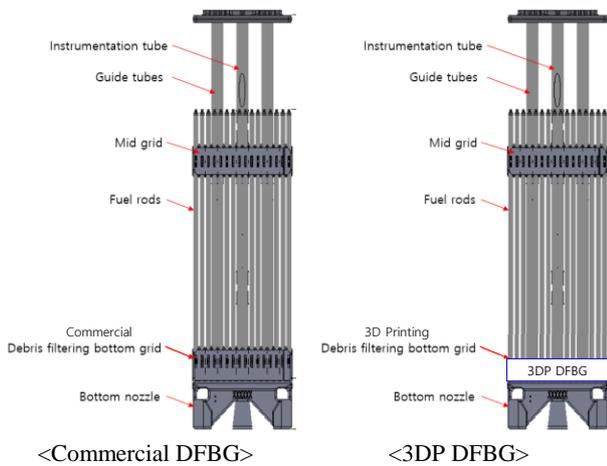
Fig. 5. Schematic of the test assembly for pressure drop
