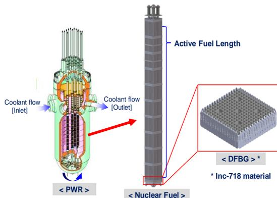
Fig. 1. General configuration of DFBG in a nuclear fuel
