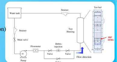
Schematic of the test facility
