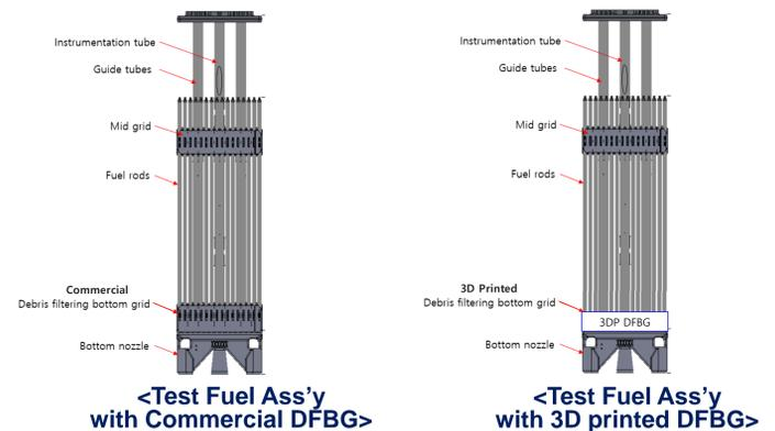
Pressure drop characteristics of 3D printed DFBG is reduced at about 16~18% in the test flow rate compared to that of commercial one.
