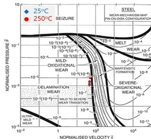
Fig. 3. Superimposition of the test results onto the wear-mode map for steel [6] (blue from 25°C test, red from 250°C)
