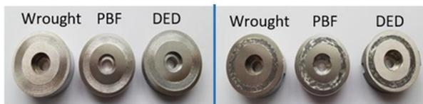
Fig. 2. Appearance of disk surface of 304L SS samples after pin-on-disk test at 25°C (left) and 250°C (right)
