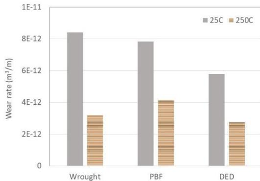
Fig. 1. Wear rates for 304L SS samples (wrought, PBF, DED) at 25 and 250°C
