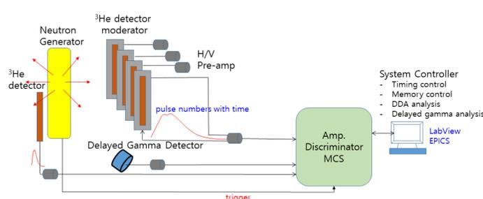
Fig. 8 Detection & Analysis scenario flowchart
