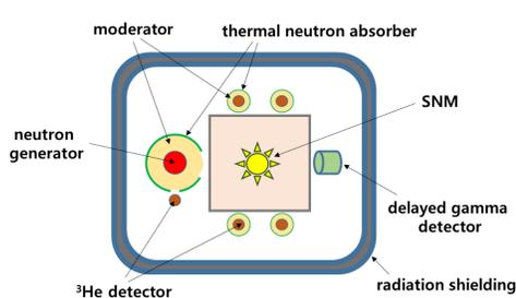
Fig. 7 Circuit diagram of the suggested DDA system
