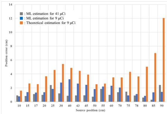
Fig. 2. ML model/theoretical position estimation error plot
