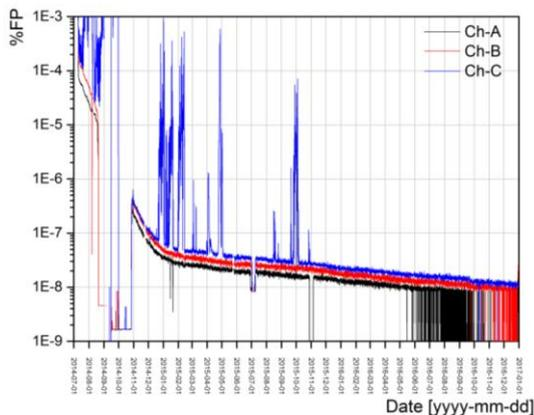
Fig. 1. Neutron power signals during the long-term shutdown of HANARO measured by RPS channel A, B and C
