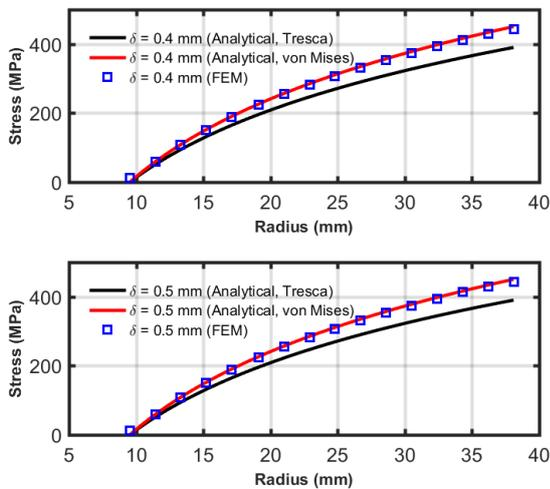
Fig. 8.  $\sigma_r$  according to  $r$  at 400 K with the free-closed end condition and  $\delta = (0.4 - 0.5)$  mm
