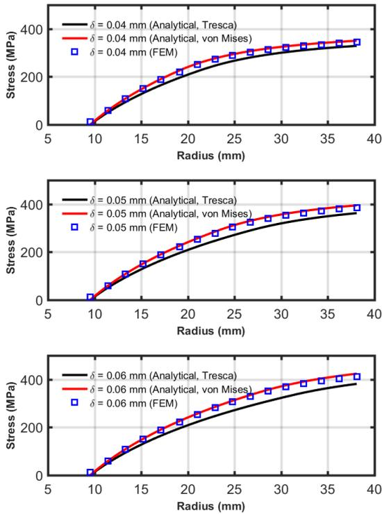
Fig. 5.  $\sigma_r$  according to  $r$  at 400 K with the free-closed end condition and  $\delta = (0.04 - 0.06)$  mm
