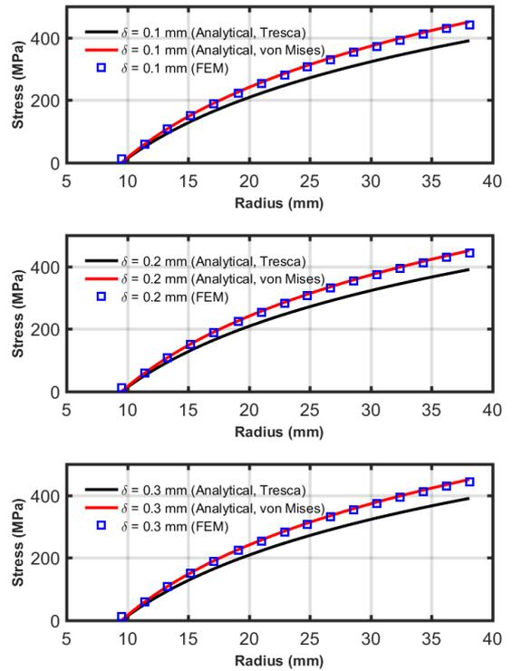
Fig. 7.  $\sigma_r$  according to  $r$  at 400 K with the free-closed end condition and  $\delta = (0.1 - 0.3)$  mm
