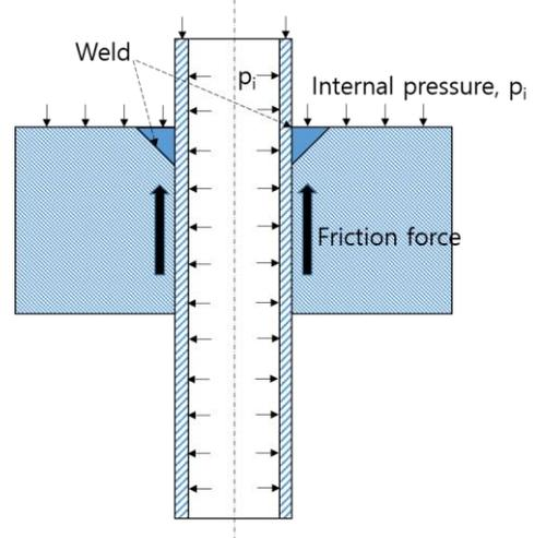
Fig. 1. Schematic of a mechanical load at a penetration area
