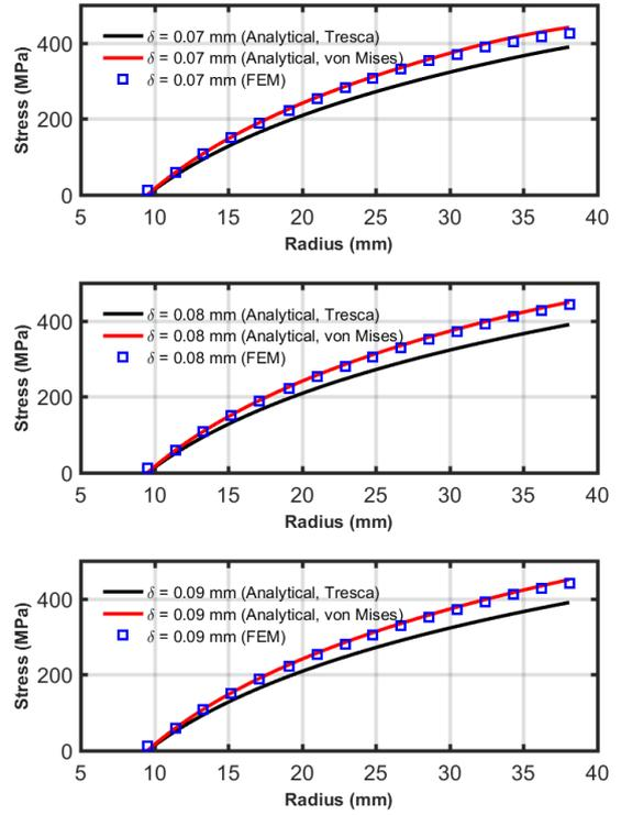
Fig. 6.  $\sigma_r$  according to  $r$  at 400 K with the free-closed end condition and  $\delta = (0.07 - 0.09)$  mm
