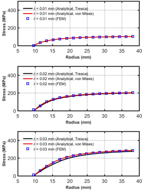
Fig. 4.  $\sigma_r$  according to  $r$  at 400 K with the free-closed end condition and  $\delta = (0.01 - 0.03)$  mm
