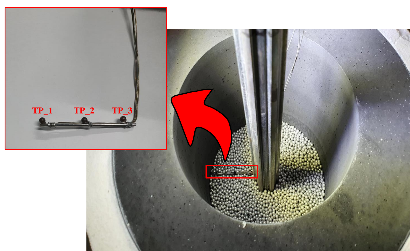
Fig. 2. Installation of thermocouples for measuring the temperature of the particles
