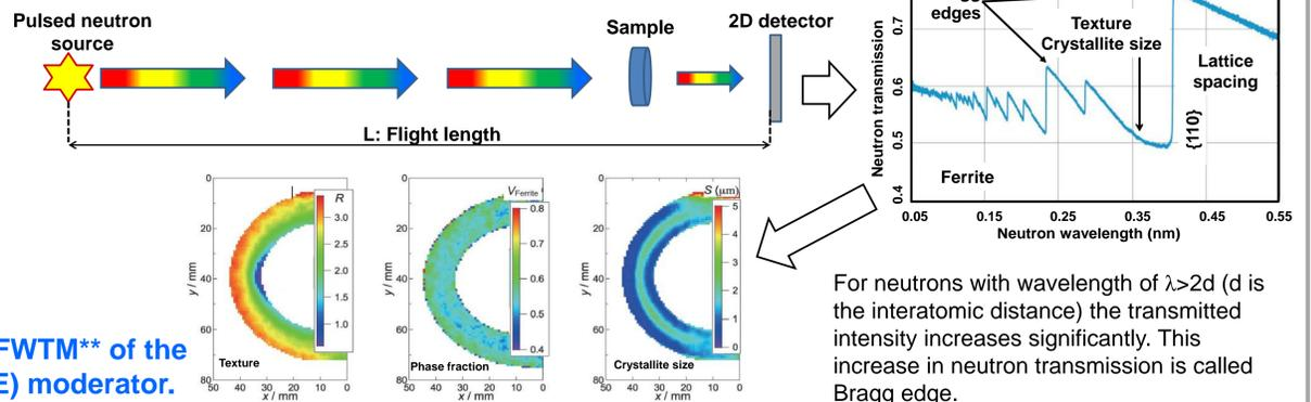
For neutrons with wavelength of  $\lambda > 2d$  (d is the interatomic distance) the transmitted intensity increases significantly. This increase in neutron transmission is called Bragg edge.
